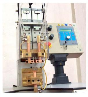
Double spot welder with indipendent electrodes: possibility to weld in sequence with an only transformer, but with distinguished control on each of the 2 electrodes or simultaneously with two generators.
